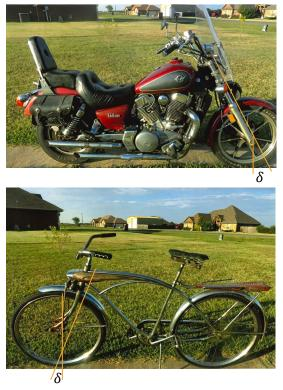
**Figure 2** (from part I): Showing the castor distance on a 1994 Kawasaki Vulcan (top) and a 1962 J.C. Higgins Flightliner (bottom). Their front wheels have been deliberately set straight ahead. All photos and images by Dwight E. Neuenschwander unless otherwise noted.
