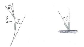
**Figure 5** (from part I): View of bike from above, showing angles  $\alpha$  and  $\eta$  and the unit vector  $\hat{n}$  (left). View of bike from behind it, showing the angle  $\theta$  (right).
