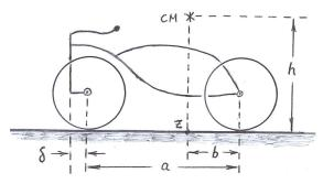
**Figure 4** (from part I): View of bike from the side, showing the distances *a*, *b*, *h*, and  $\delta$ .
