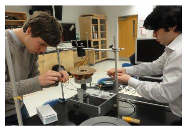
Austin and Ricardo experiment on rotating circular Halbach array - they measure a repulsive magnetic force on a coil system suspended on a force sensor.
