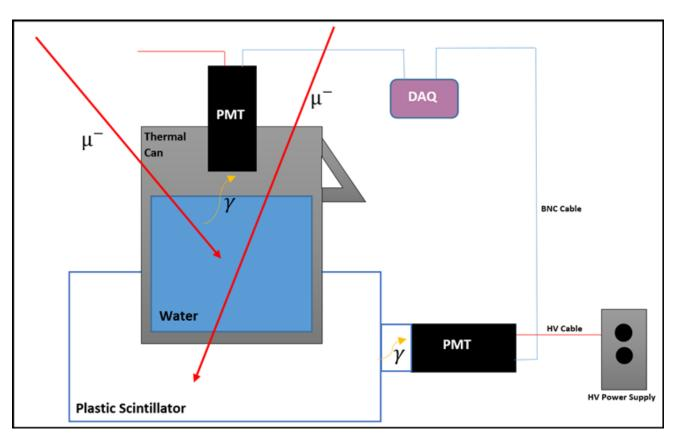
Figure 1. Diagram of the detector
