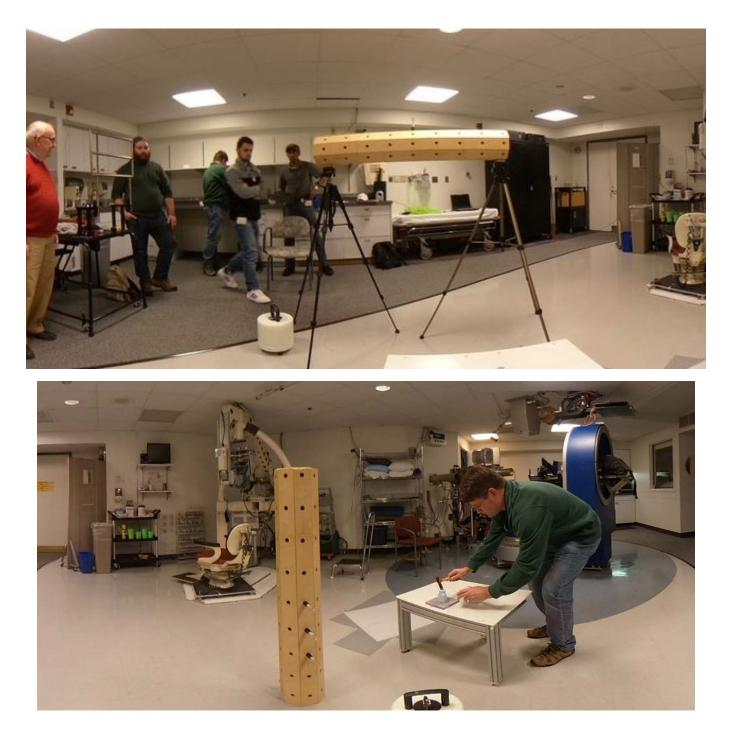
The neutron bubble detectors will be placed in a wooden stand that has 72 possible positions which was built by SPS and senior students John Thomas and Jackson Nolan, can be placed in any position, with respect to the AmBe source and the LINAC. In the above photos the array can be mounted on tripods as well as stand on its own. This array will be used to first measure a  $1/r^2$  dependence after which it can have the
