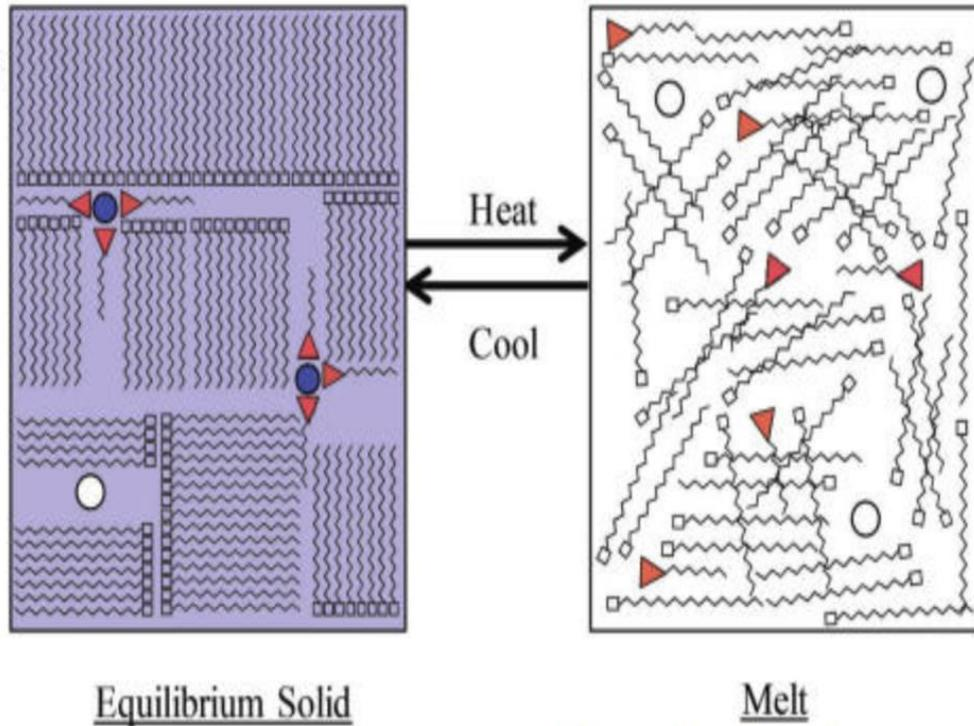
**Figure 1:** Leuco dye microstructure changes when temperature changes [10]
